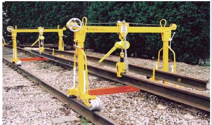
Both pairs of Ironmen experienced difficulties during braking; this resulted in them gaining speed to the point the operators could no longer control them. One of the operators of the first pair received a graze injury and another suffered from shock.
